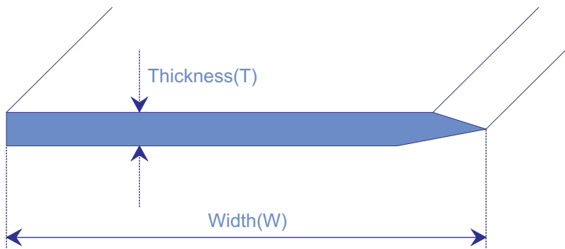
Cross section of a splitting blade
